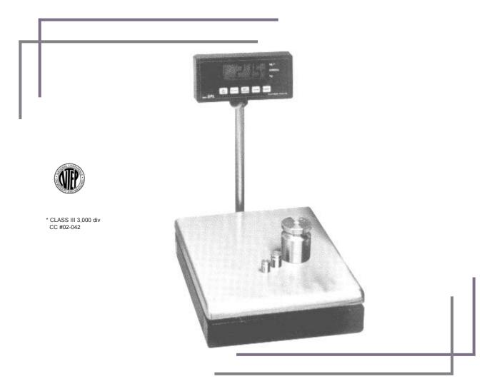
The SP Series Digital Bench Scale is an NTEP approved legal for trade, compact, 60 lb or 100 lb capacity scale with remote LED display attached with six feet of cable. An optional 12", 18", or 30" stainless steel column and mounting bracket is available. The scale features a removable stainless steel platform and adjustable feet for leveling.
