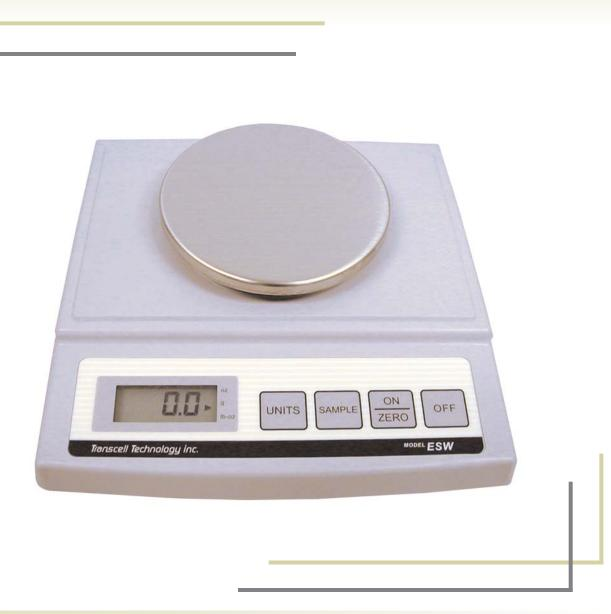
The Transcell ESW is a completely portable balance designed to stand up to the rigors of daily use, incorporating an extremely durable ABS case, an all metal sub-platter, a round stainless shroud and non-skid hard rubber feet. Precision weighing has never been easier starting with a large, LCD display, and full digital calibration. With weighing modes that include g, oz, lb-oz and parts counting, users have the versatility that is needed for a multitude of applications.
